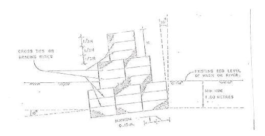
Before filling, adjacent baskets should be secured together using steel lacing wire provided for the purpose and conforming to the specification. The sides must be secured in straight lines with no gaps left between the sides of adjacent baskets. Where more than one layer of baskets is laid, they must be placed as shown on the Drawings or as directed by the Engineer with a minimum step of 0.15 m between the faces of the lower and upper gabion boxes.
